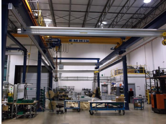
The EMH NOMAD® Free Standing Crane System and EMH Aluminum Crane Rail System (AL SYSTEMS™) work in tandem for ABB.
