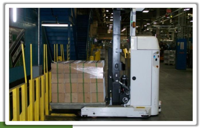
**Examples: Work-in-Process (WIP) Movement** MAVs handle the repetitive movement of materials throughout manufacturing processes.
