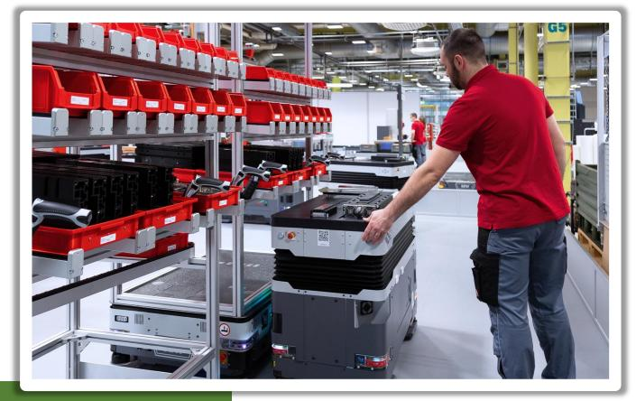
**Examples: Linking Manufacturing Cells** MAVs move products from one process to another within a production facility.
