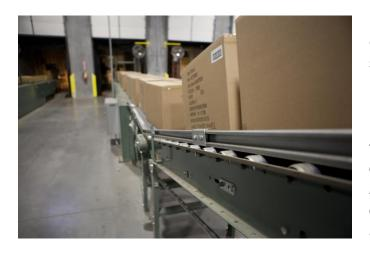
Each trailer usually represents a different destination, geographic region or carrier service; integrated scanners or imagers read the barcode or shipping label to route each parcel accordingly. As the parcels or cartons are diverted, they travel down a decline—either powered or gravity—roller conveyor (pictured left), then usually onto an accumulation conveyor (powered belt or roller) as they await loading onto the correct trailer.
