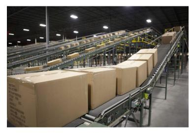
In a more automated process, the totes and cases could be transferred from an unloading conveyor to an **incline belt conveyor** (pictured left) that merges all the received items onto a single transport conveyor, either a **powered roller conveyor** or a **belt conveyor**. Depending on the size of the facility, this transport conveyor could be several hundred feet long. At the endpoint—usually a storage area—**zero-pressure**
