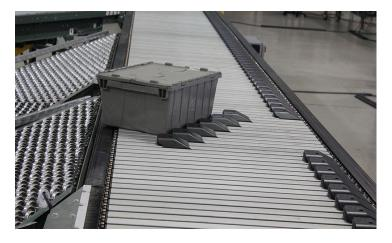
Alternately, in more automated operations, a **shoe sorter** (pictured left) could be deployed to route each item to a different destination based on identification scans. The next prestorage handling process might include manual or **in-line automatic dimensioning and weighing** (pictured below) of the received items; decanting a large box into separate items stored in totes for handling in
